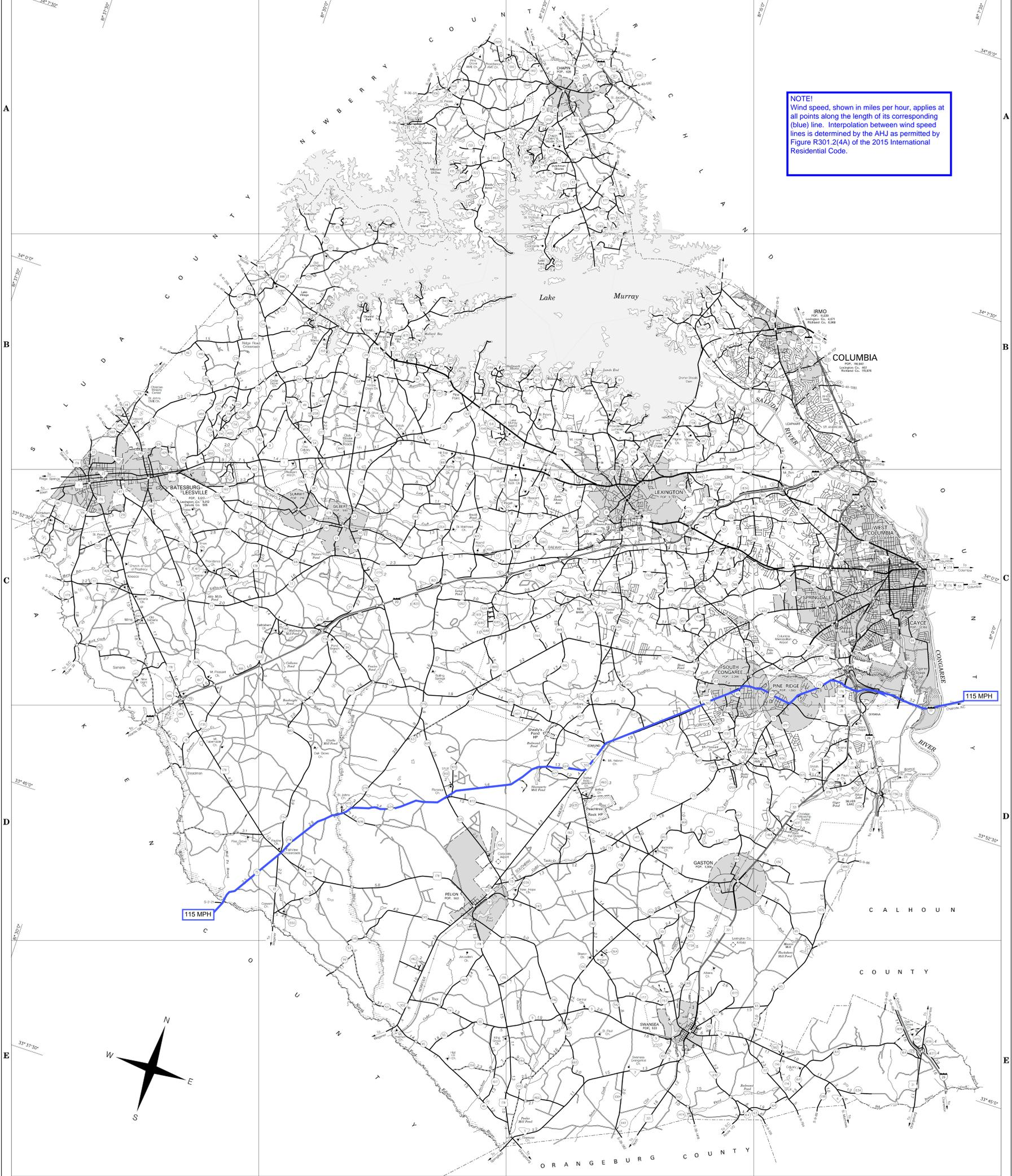
NOTE: Wind speed, shown in miles per hour, applies at all points along the length of its corresponding (blue) line. Interpolation between wind speed lines is determined by the AHJ as permitted by Figure R301.2(4A) of the 2015 International Residential Code.
