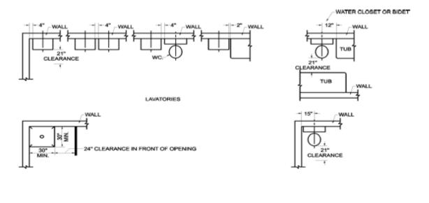
FIGURE 307.2 MINIMUM FIXTURE CLEARANCES
